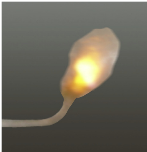
Fig. 3. Photograph of glow discharges in aqueous solution.
